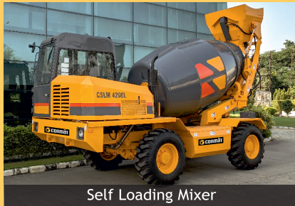
Mobile Concrete Batching Plant
